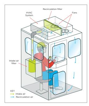
Figure 6: Filtration system for an enclosed cab
