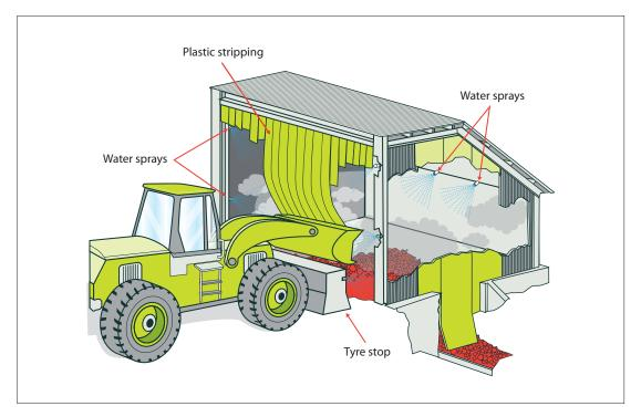
Figure 12: Example of enclosed hopper with water sprays
