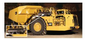
Figure 15: Diesel particulate filter
