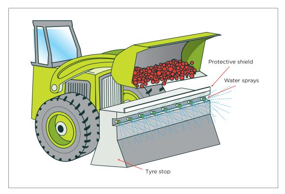
Figure 13: Example of spray bar in a concrete tyre stop
