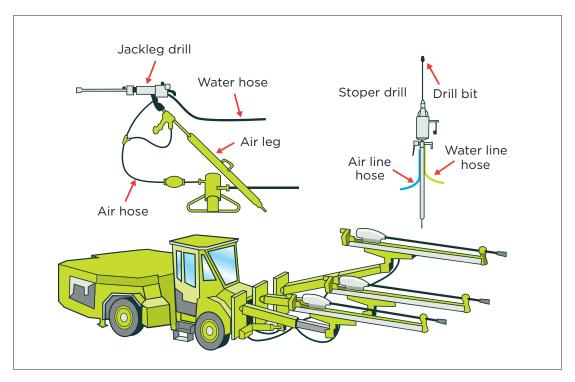
Figure 8: Wet drilling equipment
