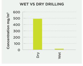
Figure 7: Reduction of dust for wet drilling
