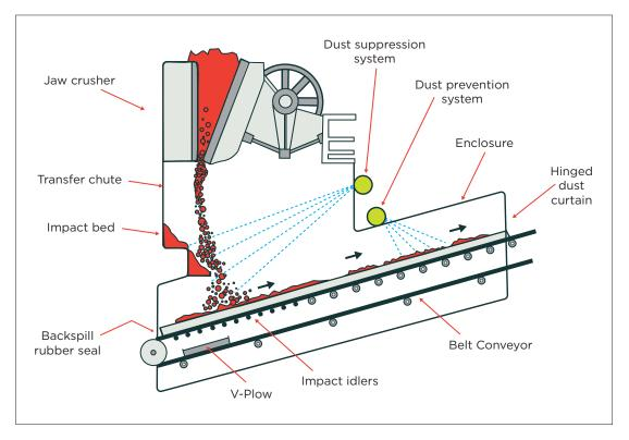
Figure 14: Example of enclosed discharge from jaw crusher with water sprays
