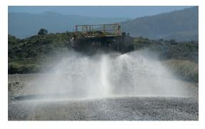
Figure 4: Dust suppression using a mobile tanker
