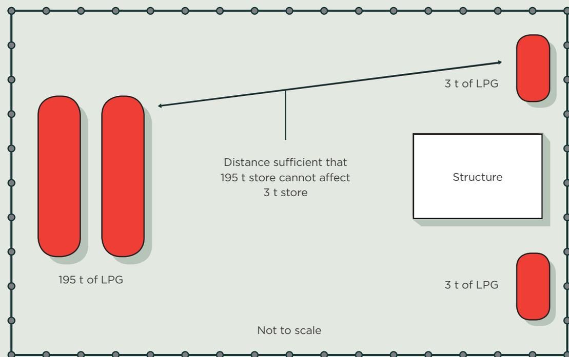
**Figure 3:** Facility with isolated small quantities
