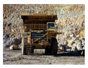
Figure 92: A stairway and platform were retrofitted to this haul truck to increase driver access and egress safety (photo courtesy of Newmont Waihi and MacMahon)
