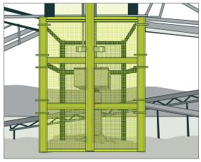
**Figure 78:** Example of perimeter guarding on gravity take-up points
