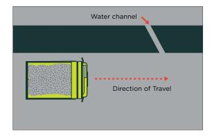
**Figure 109:** Suitable windrow - gaps in windrow for drainage
