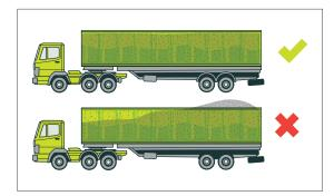
**Figure 59:** Loads should be spread evenly across the vehicle
