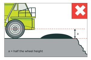
Figure 106: Unsuitable windrow - curved slopes
