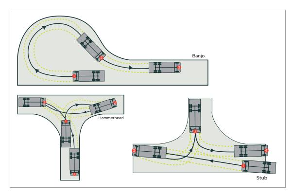
Figure 15: Turning arrangements
