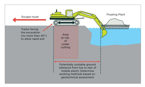
Figure 49: Excavator working beneath water, loading floating plant
