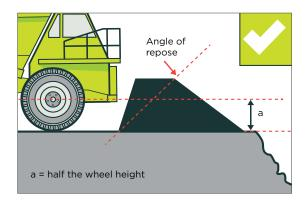
**Figure 26:** Suitable windrow - the width of the windrow is as wide as the normal angle of repose
