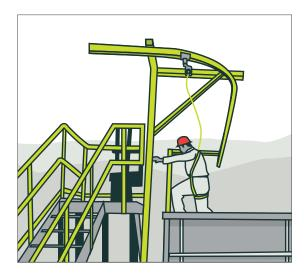
Figure 98: Overhead gantry harness system
