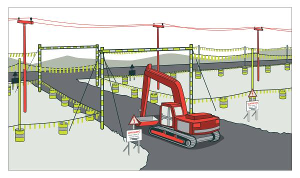
Figure 56: Safe working under overhead power lines
