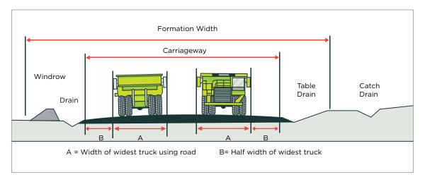
Figure 14: Example road layout with clearance between lanes
