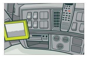
Figure 63: CCTV monitor in vehicle cab
