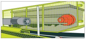
**Figure 68:** Example of close fitted guards on batch feeder belts
