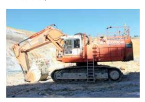
Figure 93: This excavator has a good access system, with platforms, guardrails, kick plates and ladder. The ladder is interlocked so the vehicle cannot be started without the ladder being raised (photo courtesy of Newmont Waihi and MacMahon)
