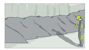
Figure 99: Example of a pedestrian windrow
