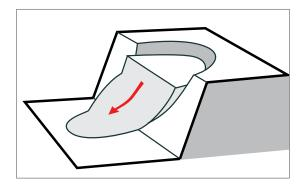
Figure 11: Circular failure
