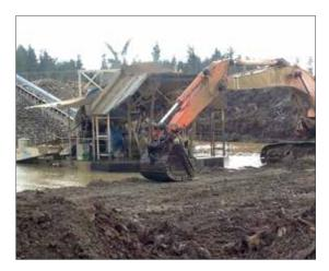
Figure 52: Digger and floating screen
