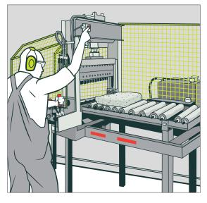
**Figure 83:** Example of two-handed starting device and drop side extraction
