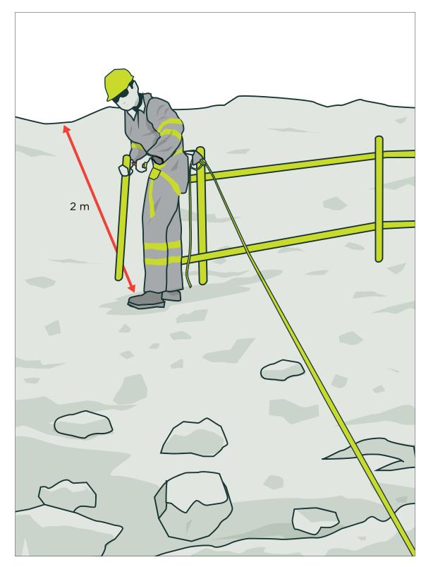
Figure 101: Example of fall restraint system
