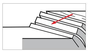
Figure 10: Toppling failure
