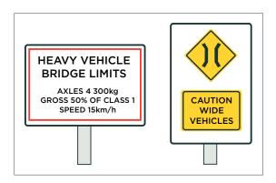
**Figure 33:** Example of weight restriction sign and narrow bridge sign
