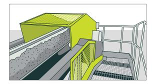
Figure 76: Example of head drum guards
