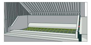
**Figure 73:** Example of steel man-grid on ground feed hopper
