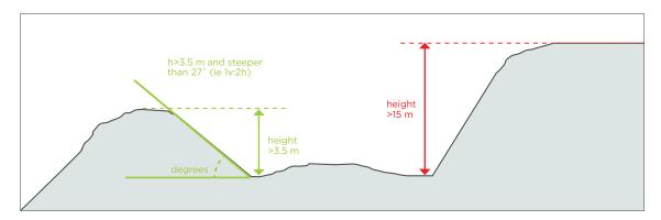
Figure 4: 'Soils and very weak rock' guidance
