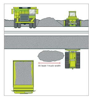
Figure 44: Vehicle separation at tip point
