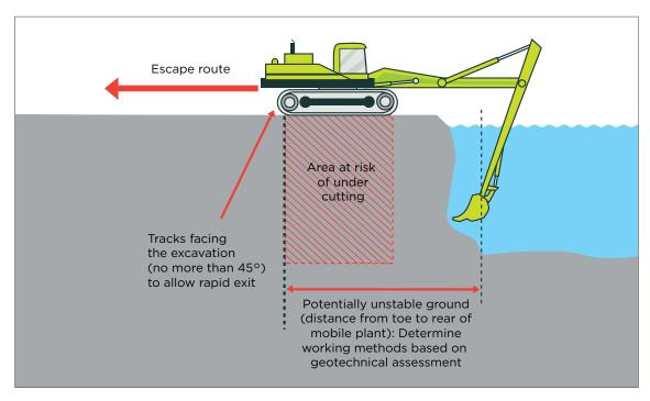
Figure 48: Long reach excavator working beneath water
