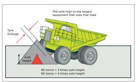
**Figure 107:** Study on windrow size to offer definite restraint
