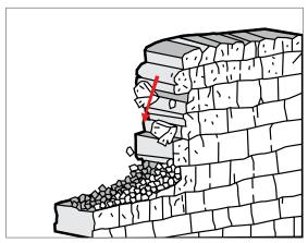
Figure 9: Ravelling failure
