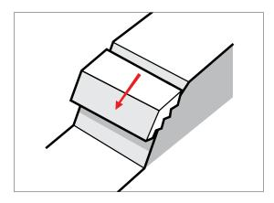
Figure 8: Step-path failure
