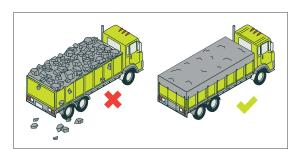
**Figure 60:** Cover loose bulk loads when travelling on a public road
