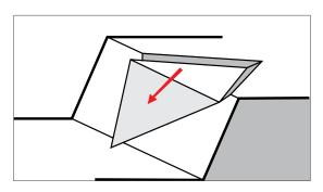
Figure 7: Wedge failure
