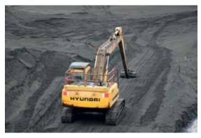
**Figure 94:** Guardrails were retrofitted to this excavator to protect workers accessing the top of the machine for maintenance purposes (photo courtesy of NZ Steel, Taharoa)
