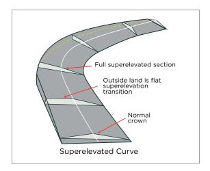
Figure 18: Superelevated bends
