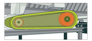
**Figure 69:** Example of close fitted guards on vee-belt drive
