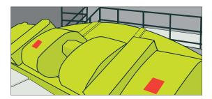
**Figure 65:** Example of totally enclosing sheet metal guard which are suitable for vibrating units with additional guards over the associated shafts and couplings
