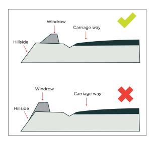
Figure 108: Windrow constructed on firm foundation
