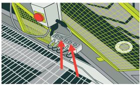
Figure 87: Example of remote greasing points
