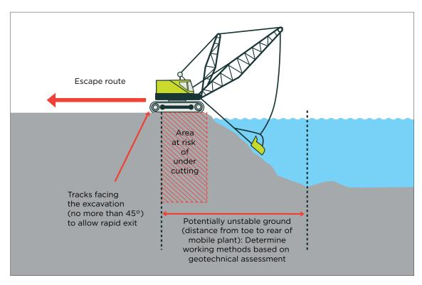
Figure 47: Dragline working beneath water
