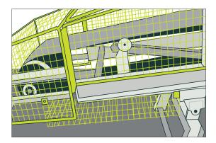
Figure 77: Example of tail drum guard
