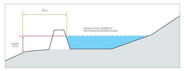
Figure 13: Guidance for tips (liquid) and ponds
