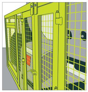
**Figure 71:** Example of hinged access panel guard bolted shut
