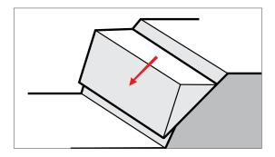
Figure 6: Planar failure
