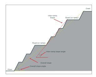
**Figure 3:** Slope design - inter-ramp and overall slope details
