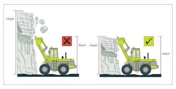
Figure 34: Face height should not exceed the reach of the loader used on the face
