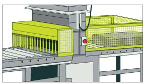
Figure 82: Stone guillotine with fixed guards
