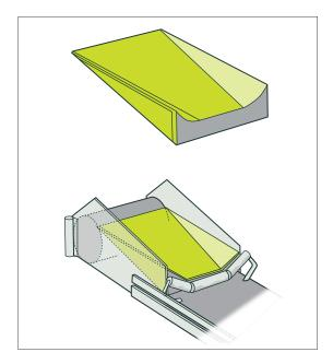
Figure 81: Head drum nip guard
