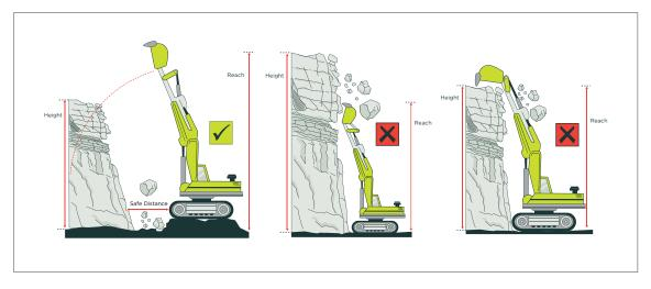
**Figure 35:** Face height should not exceed the reach of the excavator used on the face, with safe operating distances
