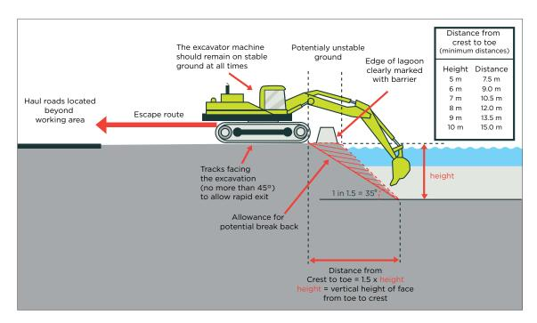
Figure 53: Example of cleaning out a settling pond with an excavator
