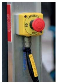
**Figure 88:** Emergency stop with signage (photo courtesy of Fulton Hogan Miner Rd Quarry and NZ Steel Taharoa)
