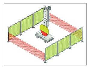
Figure 85: Stone saw with light curtains at access points
