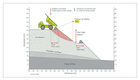
Figure 37: Example of tip slope stability design (limit equilibrium)
