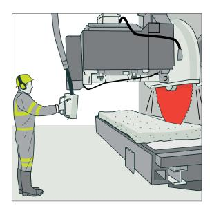
Figure 86: Remote operation controls on stone saw
