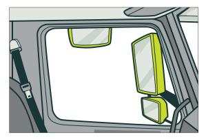
Figure 61: Side-mounted mirrors
