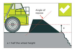
**Figure 105:** Suitable windrow – the width of the windrow is as wide as the normal angle of repose
