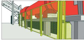
Figure 67: Example of panel type guards on dryer
