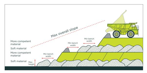
Figure 38: Example dump construction method for mixed material (mattressing)
