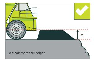
**Figure 25:** Suitable windrow – firm material big enough to absorb the vehicle's momentum with a steepened inside slope
