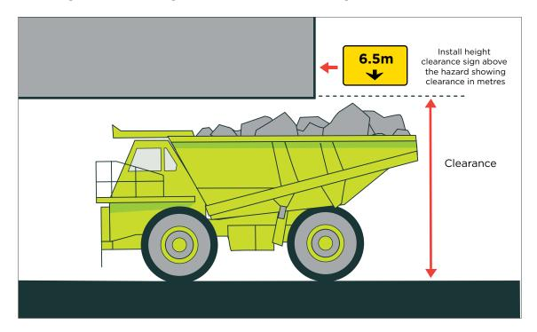
Figure 57: Example clearance signage and placement
