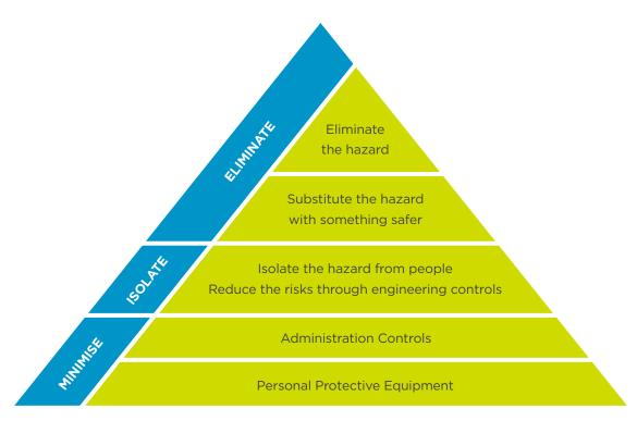
Figure 1: Hierarchy of controls
