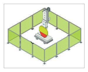
Figure 84: Stone saw with gate at access points
