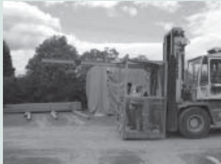
This engineer-certified forklift cage features an extended rail to which workers can attach harnesses while spreading tarps on timber stacks
