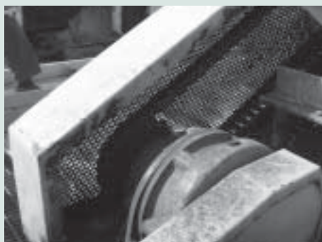
✘ Chain drive not fully guarded
