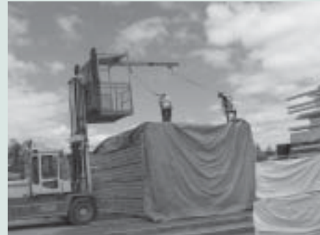
This engineer-certified forklift cage features an extended rail to which workers can attach harnesses while spreading tarps on timber stacks
