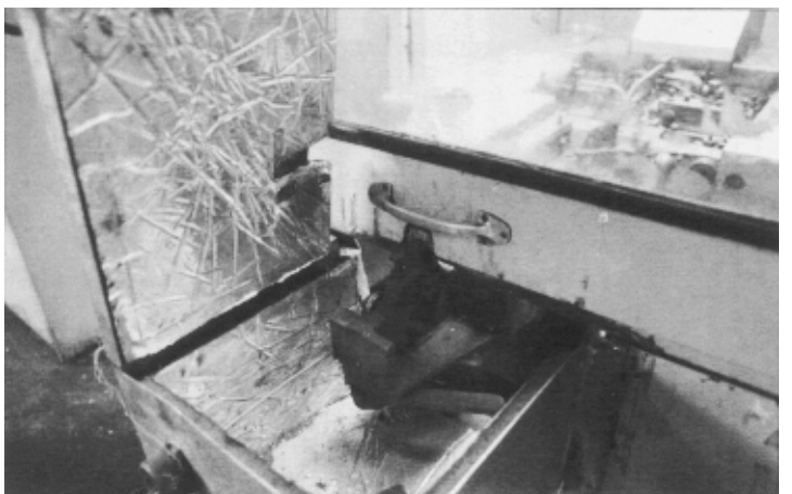
Figure 3: Silencing box fitted to the enclosure.
