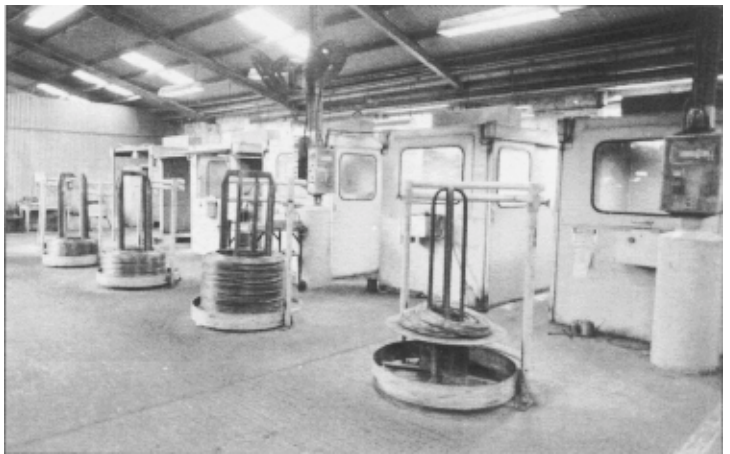
Figure 2: View of the nail making machine showing the total enclosure.
