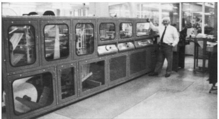
Figure 4: The glove making machine showing enclosed sides, the Venturi exhaust ducting above and the windows (in the background) of the enclosing room.
