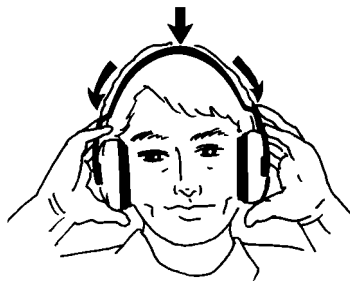
Figure 7: Tightening the headband to hold cups firmly in position
