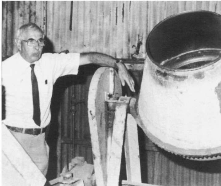
Figure 4: Nail rumbler with sound damping material painted onto the drum.
