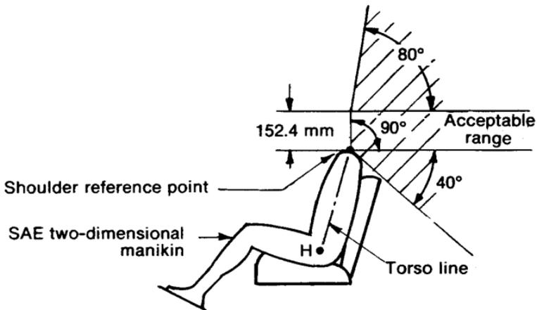
Figure 3 Anchorages for upper torso belts (see SAE J383)
