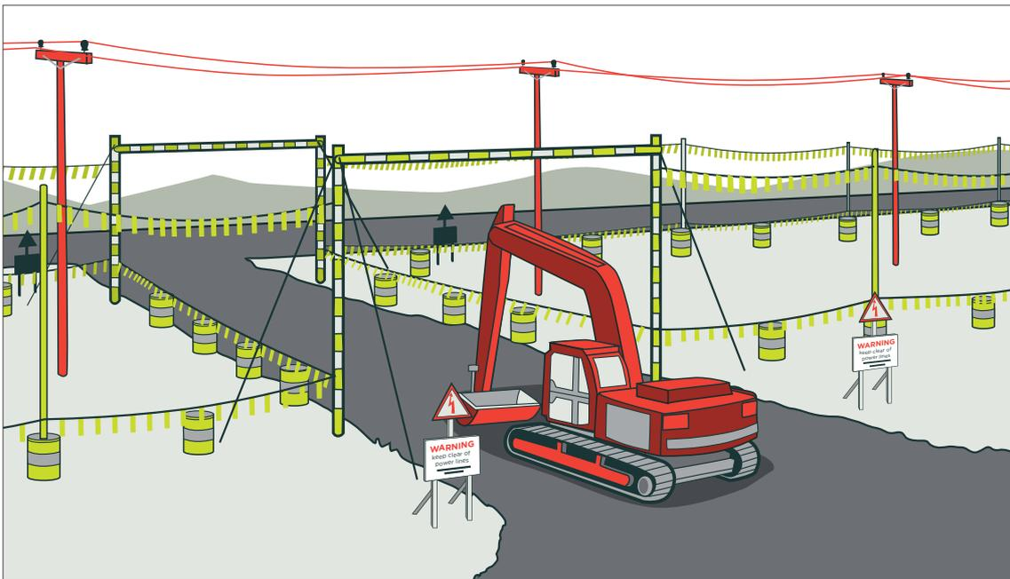
Figure 56: Safe working under overhead power lines
