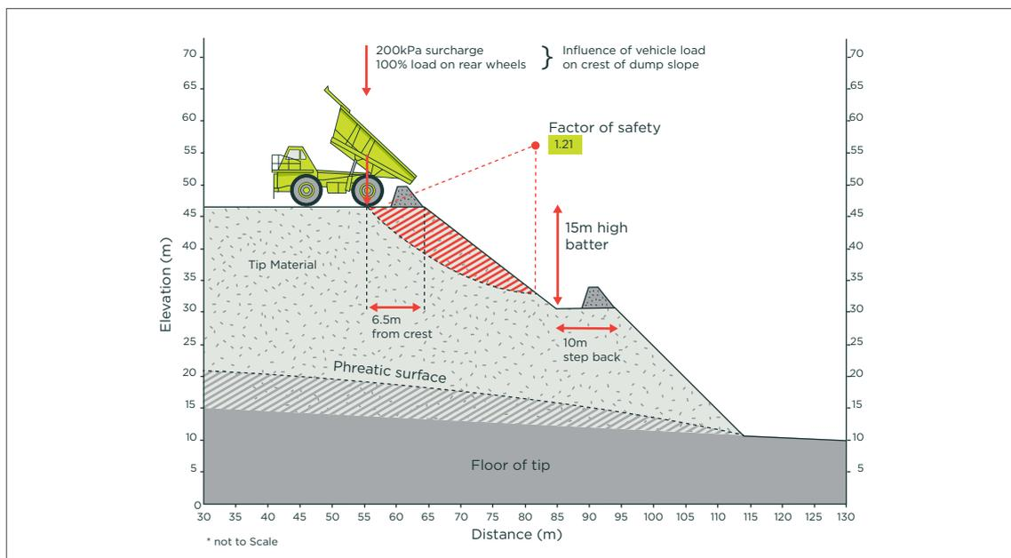
Figure 37: Example of tip slope stability design (limit equilibrium)
