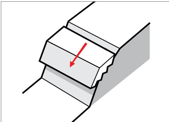
Figure 8: Step-path failure
