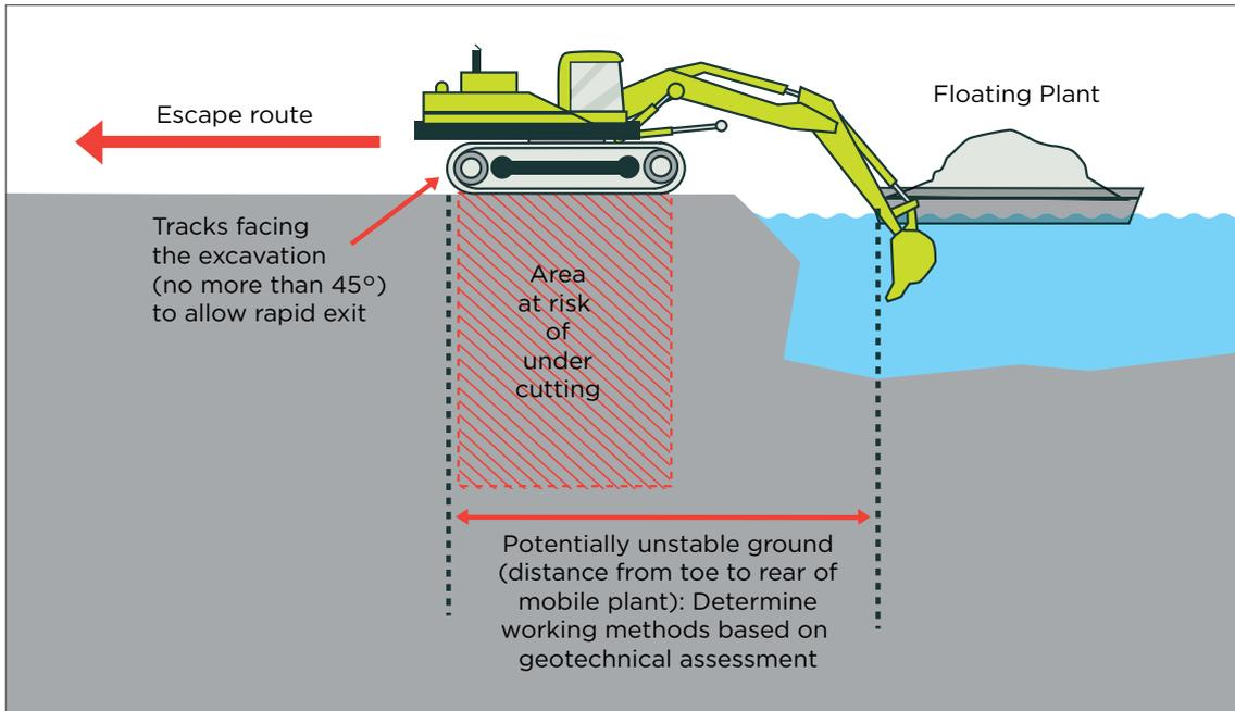
Figure 49: Excavator working beneath water, loading floating plant
