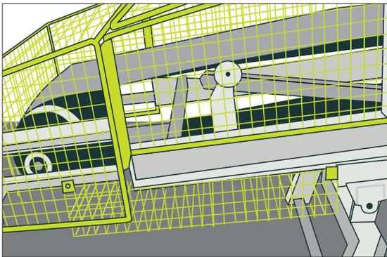
Figure 77: Example of tail drum guard
