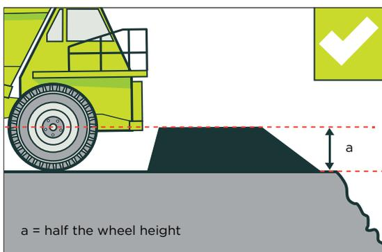
**Figure 104:** Suitable windrow - firm material big enough to absorb the vehicle's momentum with a steepened inside slope
