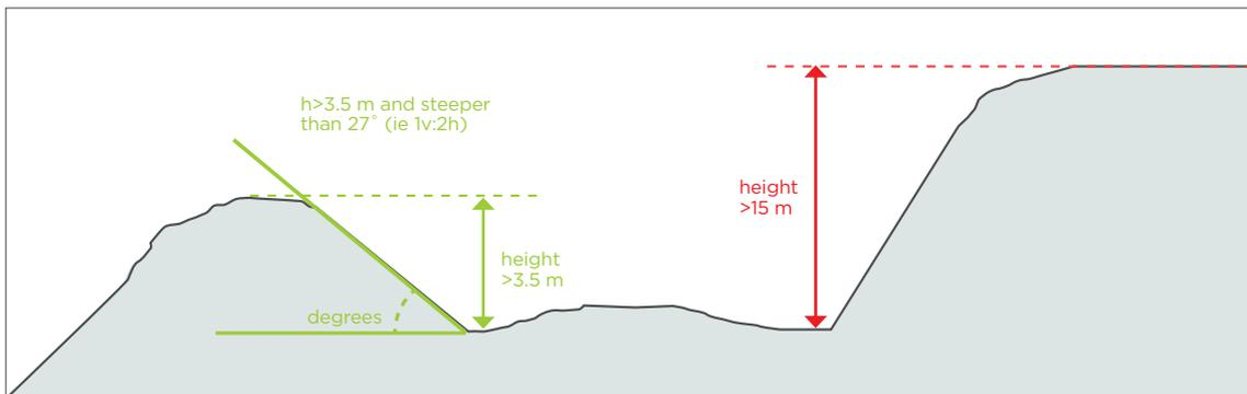
Figure 4: ‘Soils and very weak rock’ guidance
