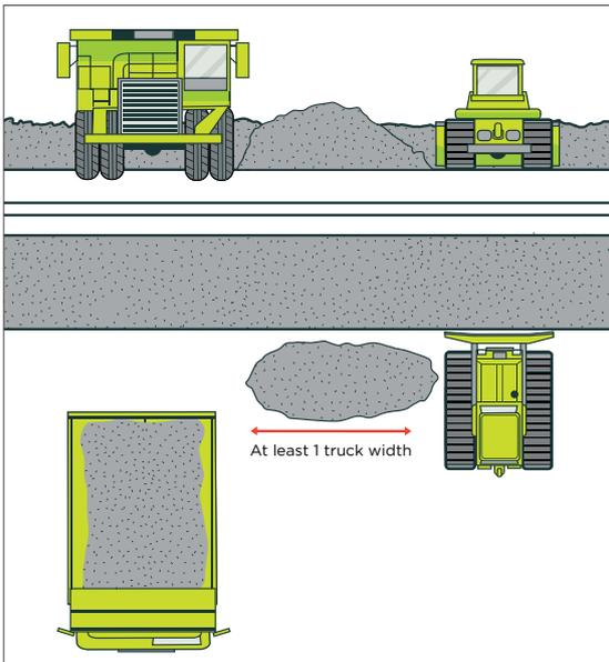
Figure 44: Vehicle separation at tip point
