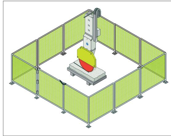
Figure 84: Stone saw with gate at access points
