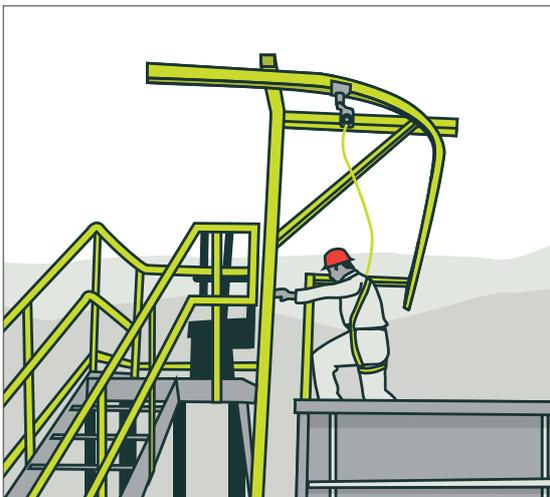
Figure 98: Overhead gantry harness system
