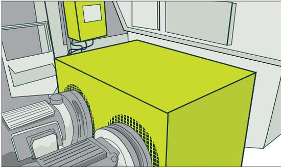
**Figure 64:** Example of fixed close-fitted guard enclosure on direct drive electric motors
