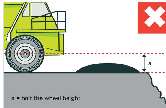
**Figure 106:** Unsuitable windrow - curved slopes
