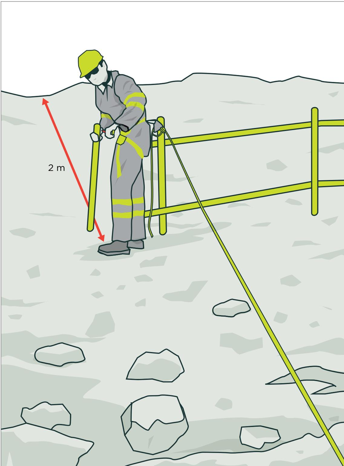
Figure 101: Example of fall restraint system
