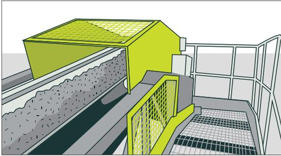
Figure 76: Example of head drum guards
