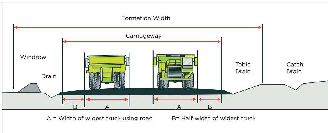
Figure 14: Example road layout with clearance between lanes
