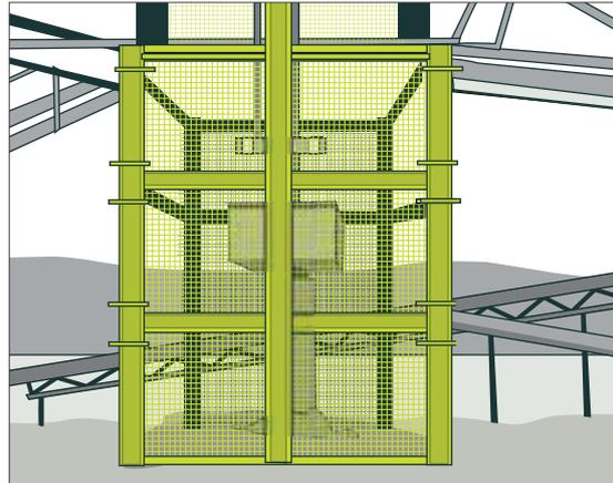
Figure 78: Example of perimeter guarding on gravity take-up points
