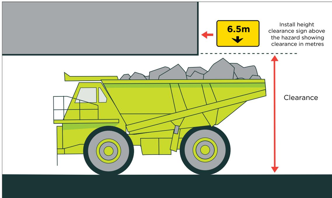
**Figure 57:** Example clearance signage and placement
