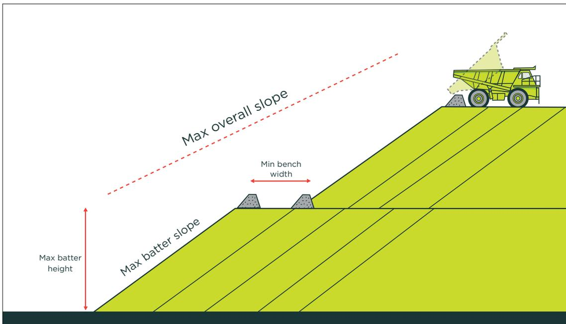
Figure 39: Example dump construction method for competent material
