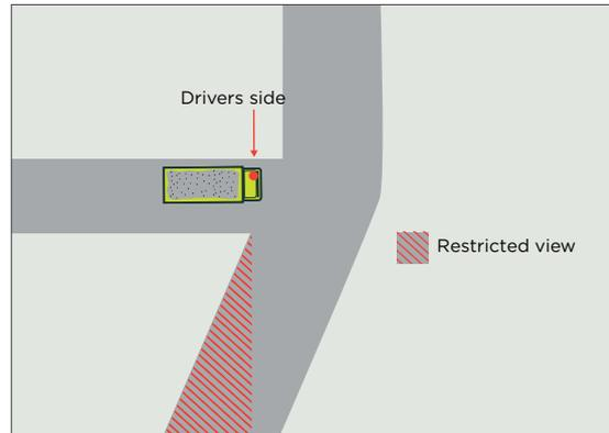
Figure 21: Intersection with restricted view
