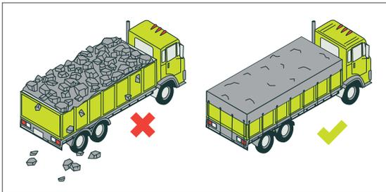
**Figure 60:** Cover loose bulk loads when travelling on a public road
