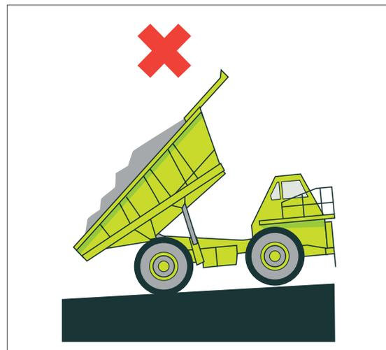
**Figure 43:** Dump on level ground with a slight uphill gradient
