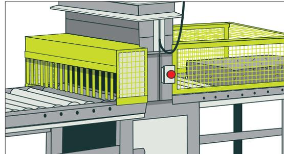
Figure 82: Stone guillotine with fixed guards
