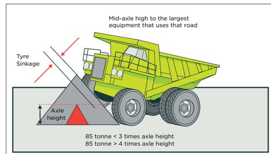
**Figure 107:** Study on windrow size to offer definite restraint
