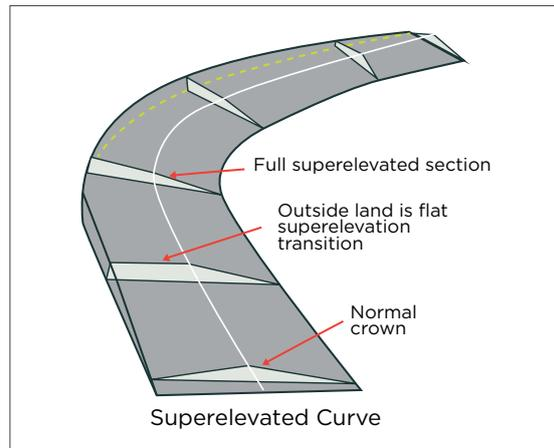
**Figure 18:** Superelevated bends
