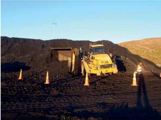
Figure 103: Vehicle overturn emergency
