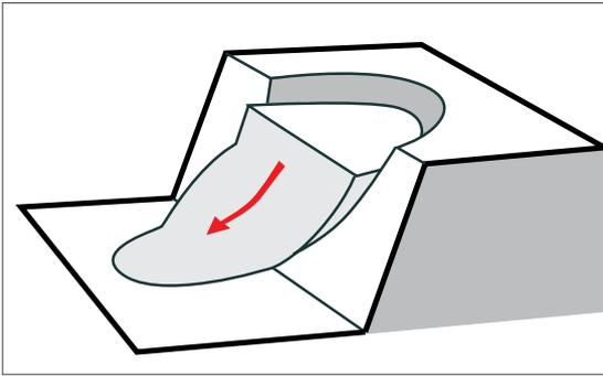
Figure 11: Circular failure
