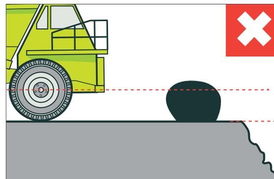
**Figure 28:** Unsuitable edge protection – blocks of stone can be pushed out of the way
