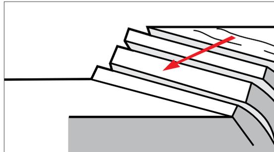
Figure 10: Toppling failure
