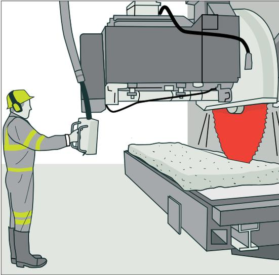
Figure 86: Remote operation controls on stone saw
