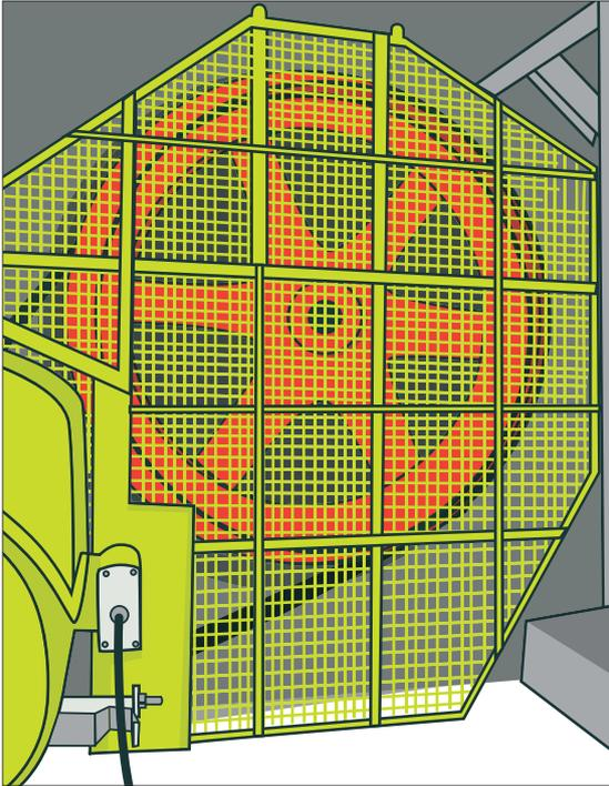
**Figure 70:** As with vee belt drives, a fixed guard totally enclosing the drive is suitable for primary jaw crusher drives. Alternatively guarding fitted around existing structures may be suitable
