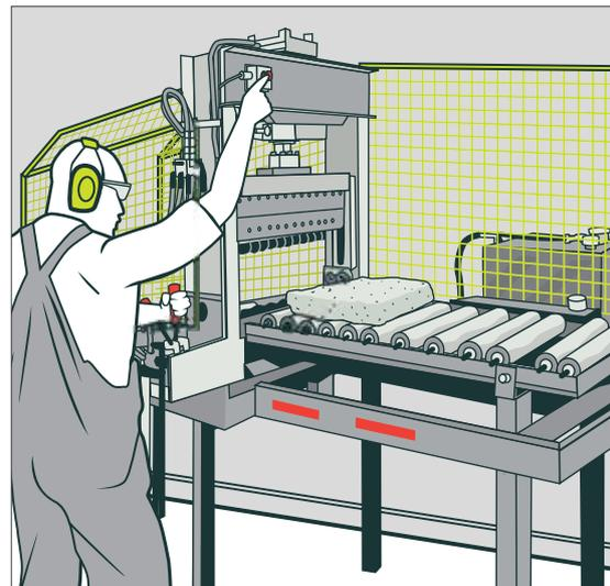
Figure 83: Example of two-handed starting device and drop side extraction
