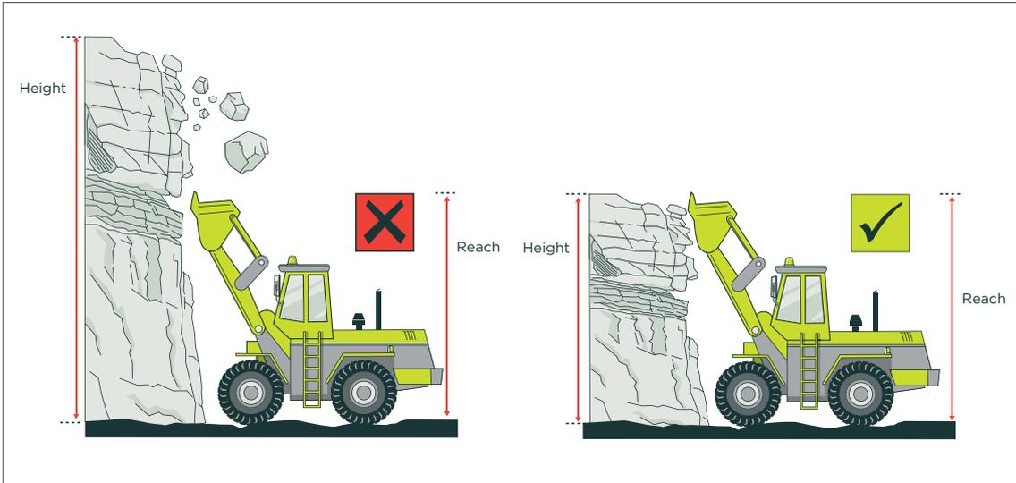
Figure 34: Face height should not exceed the reach of the loader used on the face
