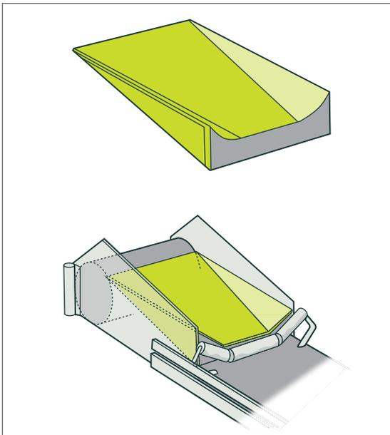
Figure 81: Head drum nip guard
