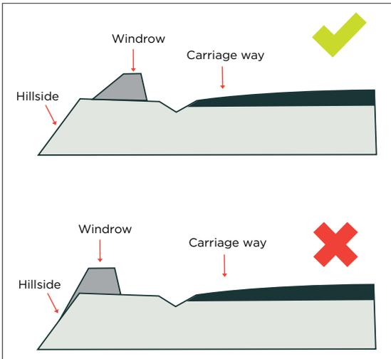
**Figure 108:** Windrow constructed on firm foundation
