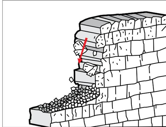
Figure 9: Ravelling failure
