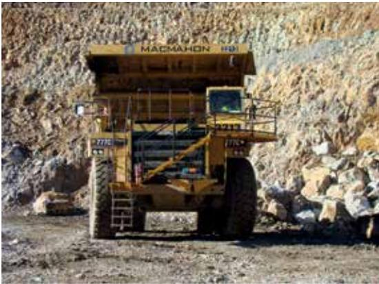
**Figure 92:** A stairway and platform were retrofitted to this haul truck to increase driver access and egress safety (photo courtesy of Newmont Waihi and MacMahon)
