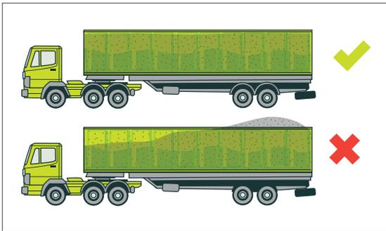
**Figure 59:** Loads should be spread evenly across the vehicle
