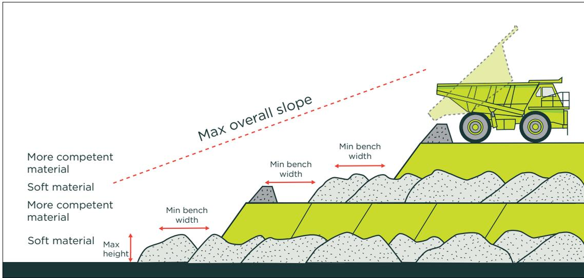
Figure 38: Example dump construction method for mixed material (mattressing)
