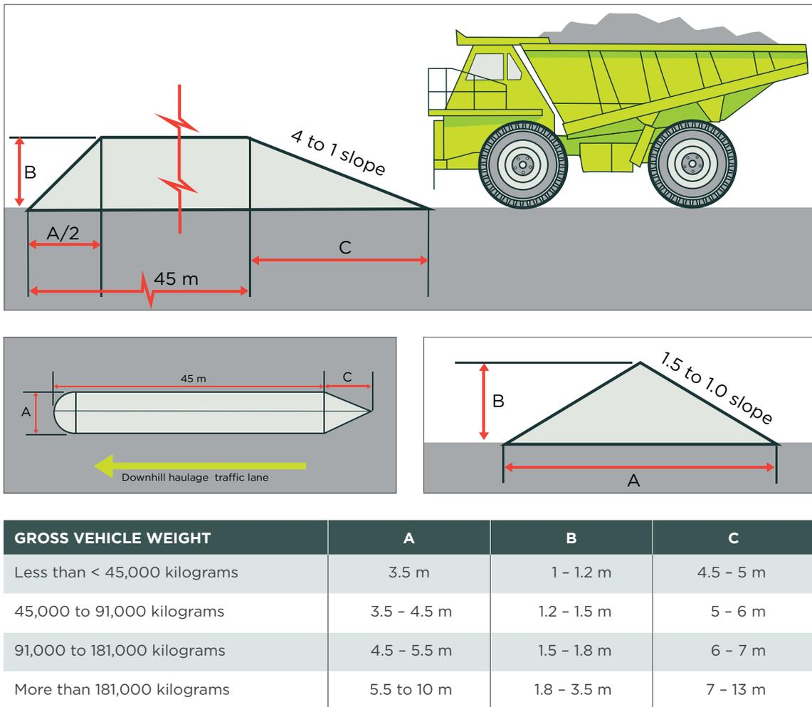
Figure 29: Runaway-vehicle centre berm
