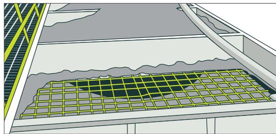
**Figure 72:** Example of steel man-grid on elevated feed hopper
