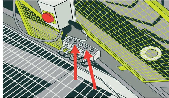
Figure 87: Example of remote greasing points
