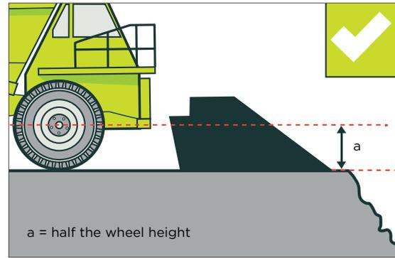
**Figure 27:** Suitable edge protection – a rock with material in between which can safely absorb the impact
