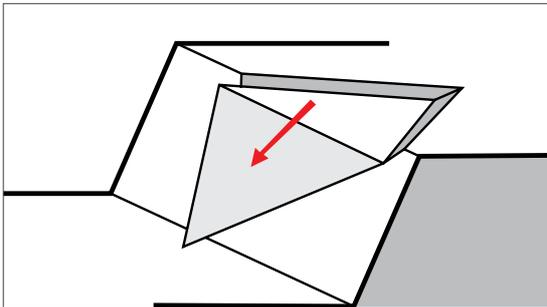
Figure 7: Wedge failure
