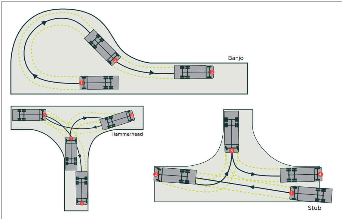
Figure 15: Turning arrangements
