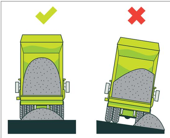
**Figure 42:** Vehicles should be parked on level ground (side to side) when dumping their load
