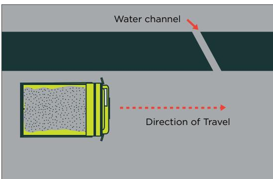
**Figure 109:** Suitable windrow – gaps in windrow for drainage
