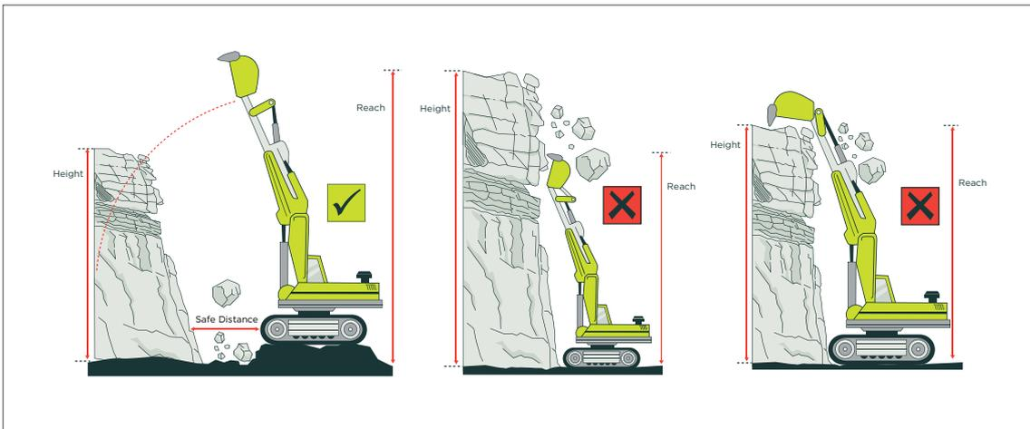
Figure 35: Face height should not exceed the reach of the excavator used on the face, with safe operating distances
