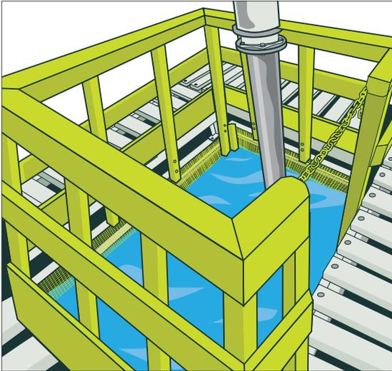
**Figure 51:** Example of guardrails around a water pick-up station
