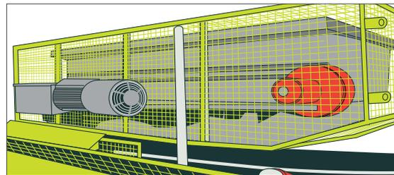
**Figure 68:** Example of close fitted guards on batch feeder belts
