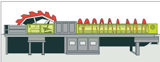
**Figure 66:** Example of panel mesh guards on fines dewaterer
