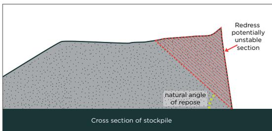
Figure 46: Cross section of stockpile
