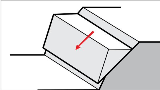
Figure 6: Planar failure
