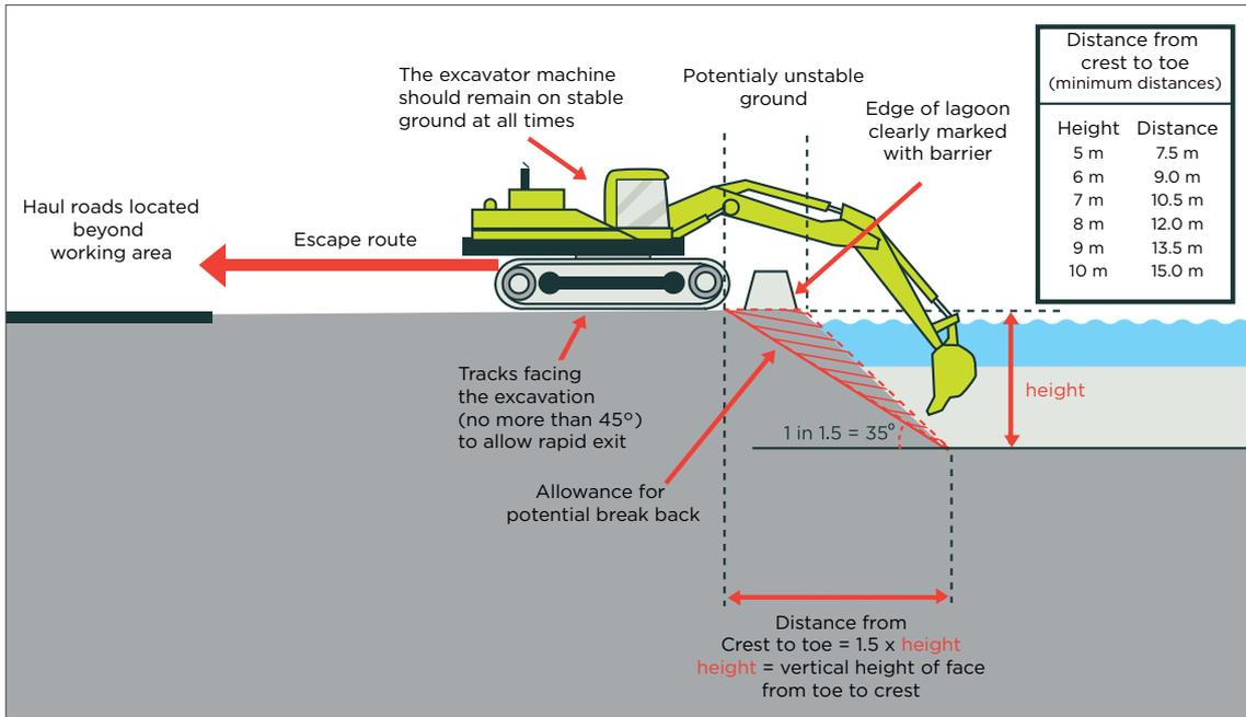
Figure 53: Example of cleaning out a settling pond with an excavator
