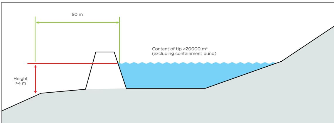
Figure 13: Guidance for tips (liquid) and ponds
