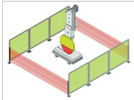
Figure 85: Stone saw with light curtains at access points
