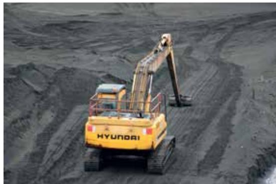
**Figure 94:** Guardrails were retrofitted to this excavator to protect workers accessing the top of the machine for maintenance purposes (photo courtesy of NZ Steel, Taharoa)
