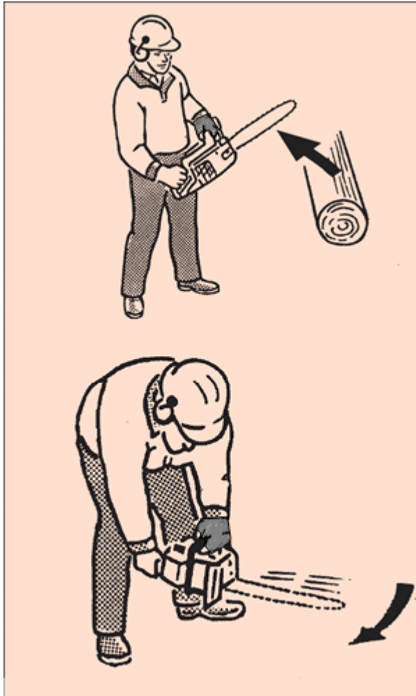
Fig 9: Inertia chainbrake triggers brake in any position when kickback occurs.
