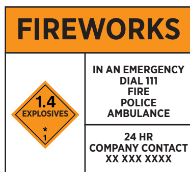
FIGURE 5: Sample sign for fireworks and safety ammunition
