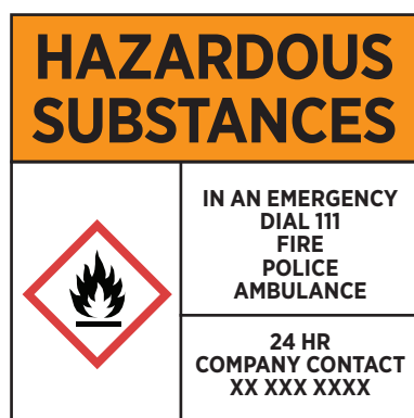
FIGURE 2: Sample sign for substances in a building (but not a dedicated room/compartment)
