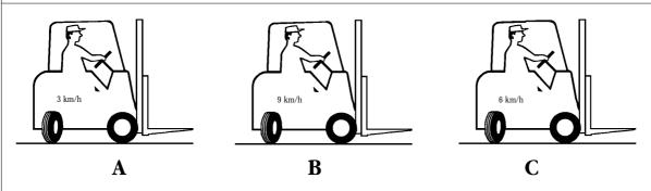
**6.** These short-based forklift trucks are turning at full lock. The forward speed is 3 km/h, so the rear end swing will travel at?
