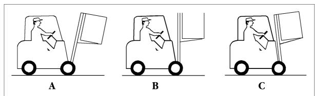
13. Each load contains 1 tonne evenly distributed. Which forklift truck has most weight on its back wheel?
