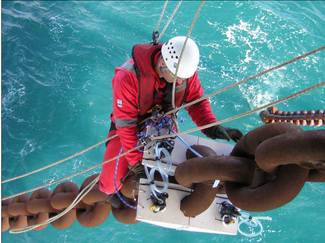
Figure 2: Abseiler on ship's chain undertaking a test run for cutting anchor chains on floating oil and gas vessel, offshore Taranaki. Photo by DJ Matheson.
