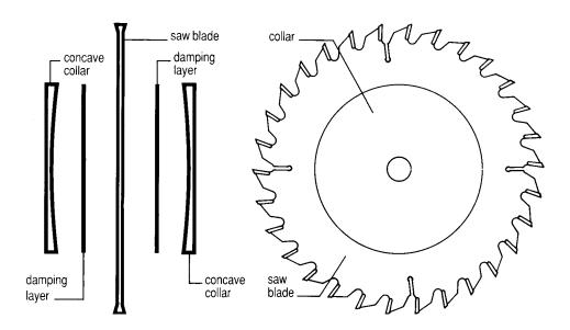
Fig. 6 Design of vibration damping collars
