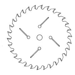
Fig.2 Deep slots in saw blade
