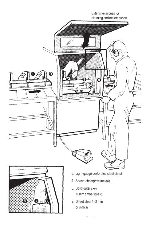
Fig. 8 Examples of materials for enclosure
