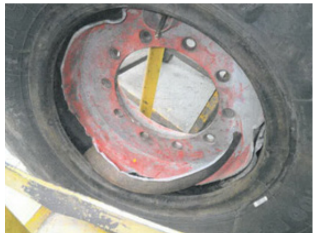
FIGURE 2: Rim damage after explosion
