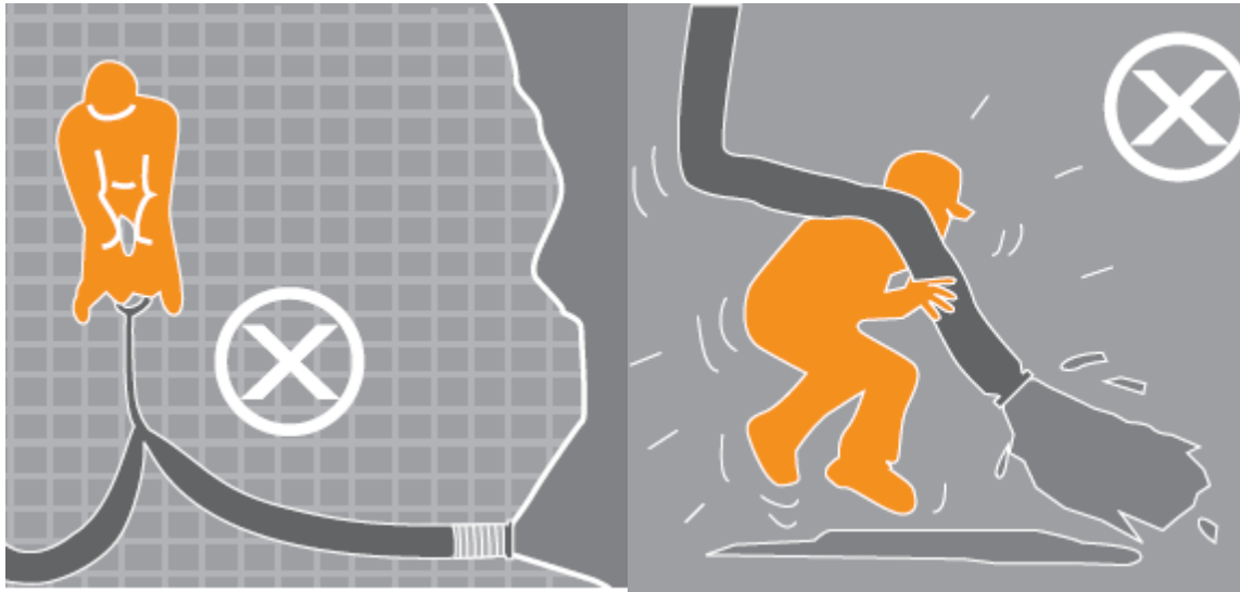
Figure 14: Do not allow hose to kink
