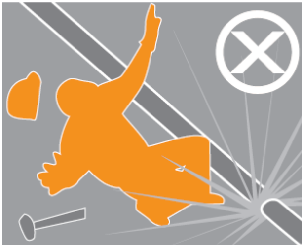
Figure 18: Never dismantle pipeline while under pressure
