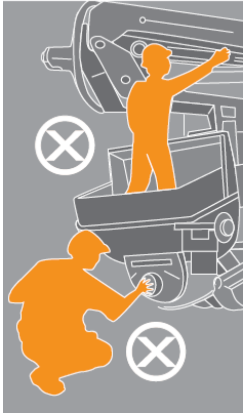
Figure 20: Dangerous cleaning practices
