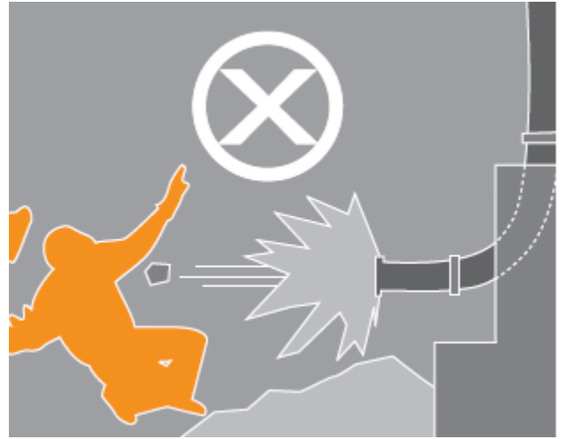
Figure 17: Keep clear of discharge end of pipe
