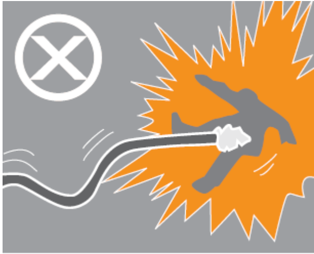
Figure 16: The end-hose should be secured or removed
