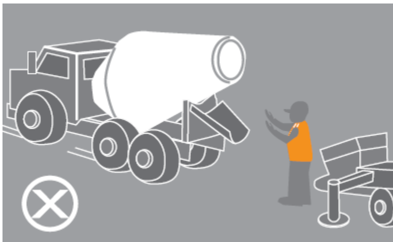
Figure 8: Keep clear when truck is reversing into position - don't stand between the truck and hopper
