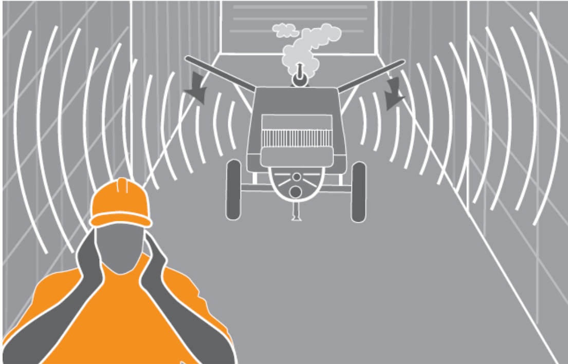
Figure 4: Beware of hazards when set up in enclosed areas
