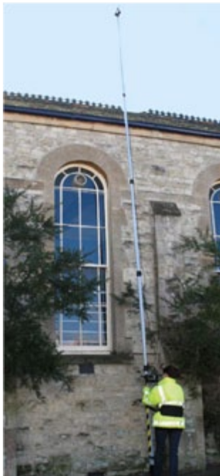
Figure 1: Remote inspection mast with hand-held lightweight CCTV system (Image courtesy of Survey Support Ltd) UK.
