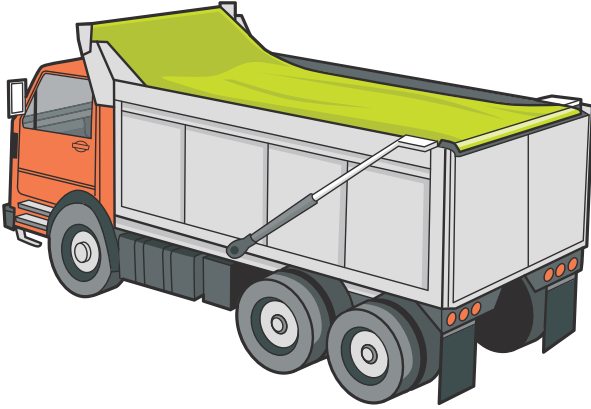
FIGURE 12: Truck with automated tarping cover
