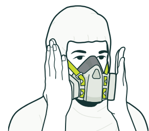
FIGURE 11: Negative-pressure fit check procedure
