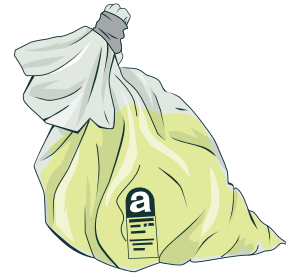
FIGURE 13: Asbestos waste bag tied with a gooseneck twist
