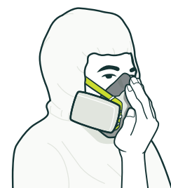
FIGURE 12: Positive-pressure fit check procedure
