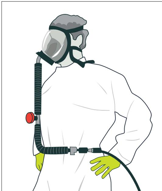
**Figure 24:** Full-face, positive-pressure demand air-line respirator
