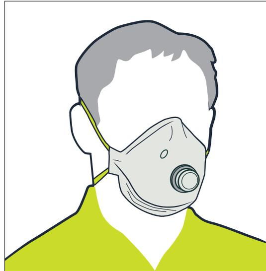
**Figure 19:** P2 half-face particulate respirator
