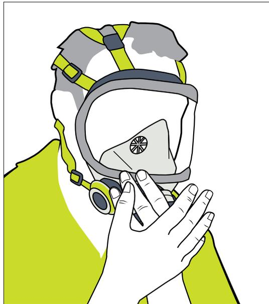
Figure 18: Conducting a fit check
