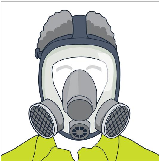
Figure 22: Full-face, particulate filter (cartridge) respirator
