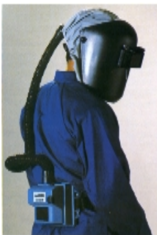
A powered positive pressure respirator has a battery powered fan or blower which draws air through the filter to the facepiece or hood. Devices with the blower unit and filter incorporated into a helmet are also available.
